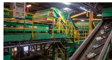
Sortation equipment separates cups, cans, containers and bottles from paper. An eddy current sorts aluminum into a metals-only stream.
